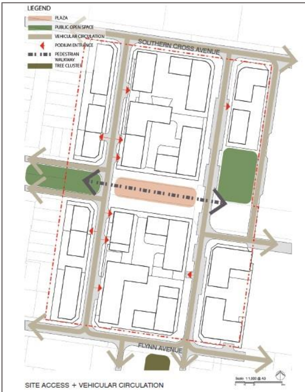
Figure 10: Site access and circulation concept (Source: Middleton Grange Urban Design Report, 26 November 2015, Urbis )
